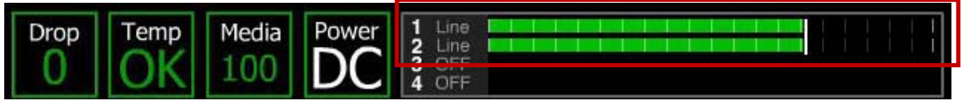
Peak Level Meter response to 0dBu (-20dBFS) Reference Level
