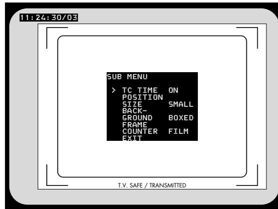
**Note:** The frame information (the last two digits of the time code display) is only active if time code is actually recorded on film. If there is no time code recording on film because for example the camera is not running on a time code speed, only the symbol "\*\*\*\*" is displayed on that position.
