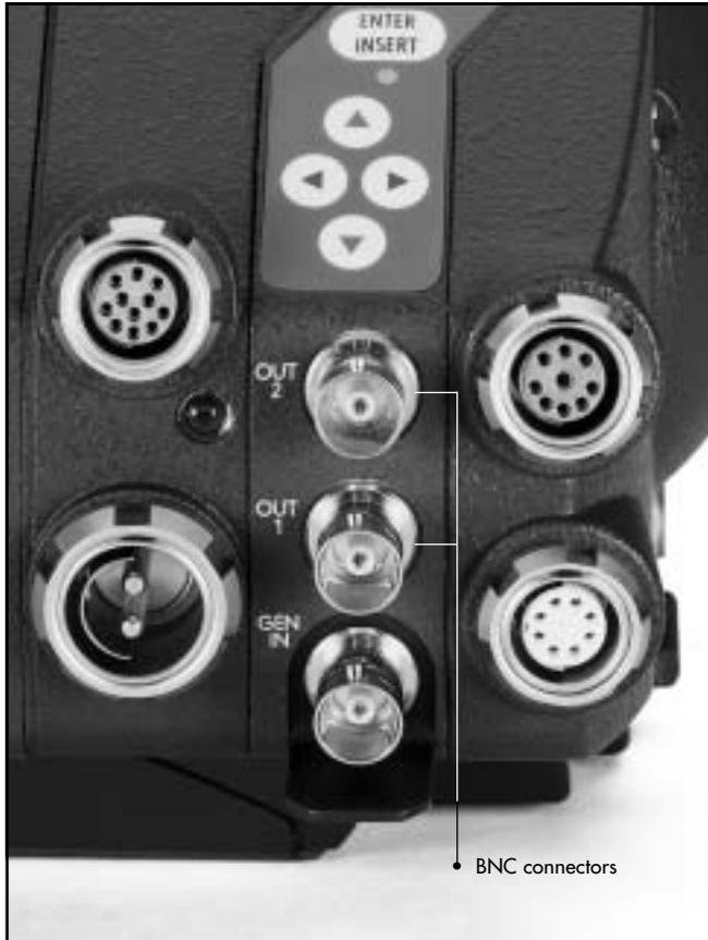
Alternatively, the Y/C signal can be taken from the two BNC outputs on the rear side of the IVS.
