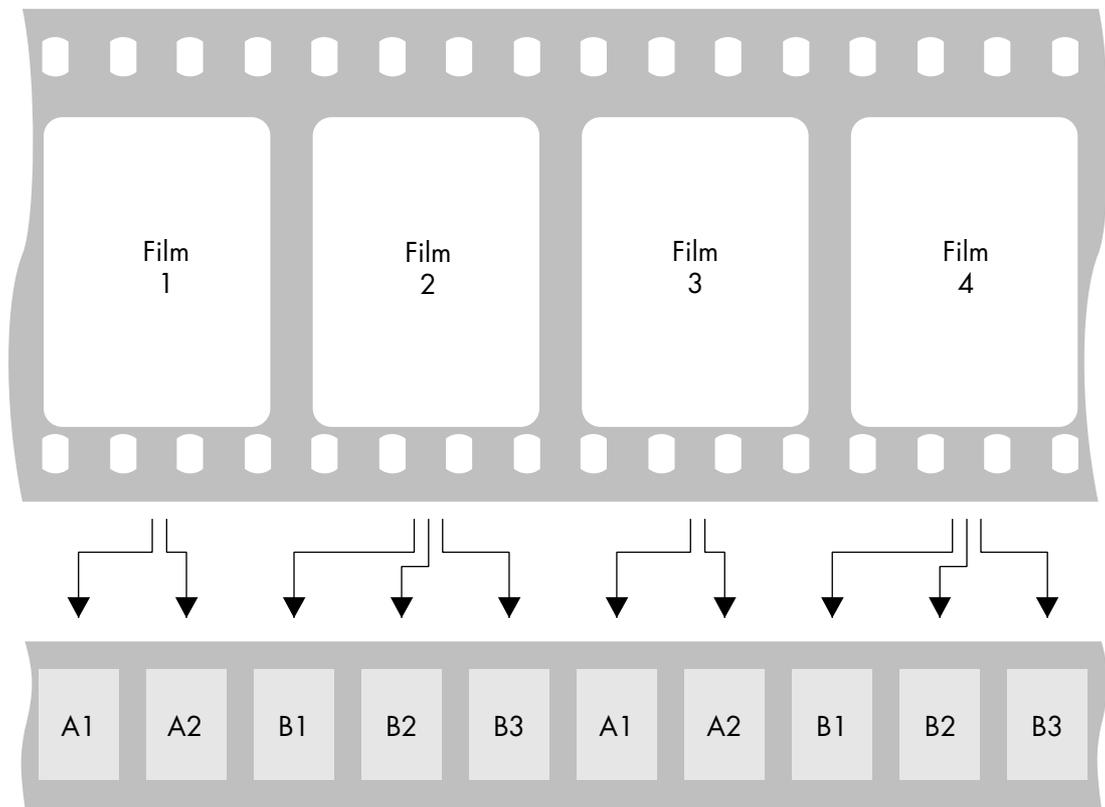
All video assists are based either on PAL or NTSC video systems, with a fixed video frequency of either 25 full video frames per second with PAL or 29.97 full video frames per second with NTSC. The speed of the film camera on the other hand can be selected over a wide range. At every film speed which is different from the video frequency, the IVS has to add repeated video fields to compensate for the different frame rates.
