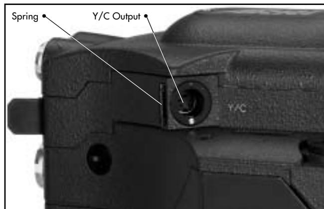
Note: This cable is secured by a spring ⇨ **photo**. To release, please press the spring and pull the cable out.
