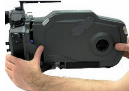
Don't forget to lock the magazine by pushing the magazine upper lock lever.
